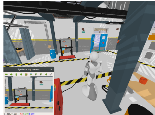
Fig. 3: Synthetic RGB image retrieval from the top camera of a virtual Pepper, in a simulated environment. The obtained RGB image is displayed in the bottom left corner, using OpenCV.
