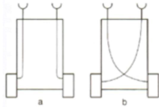
Figure 1: two simple Braitenberg vehicles
